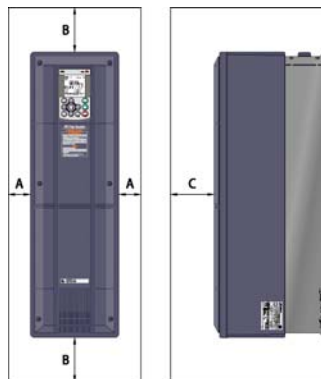
Figure 2.1 Mounting Direction and Required Clearances
