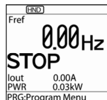
Figure 4.2 Display of the LCD Monitor after Power-ON
